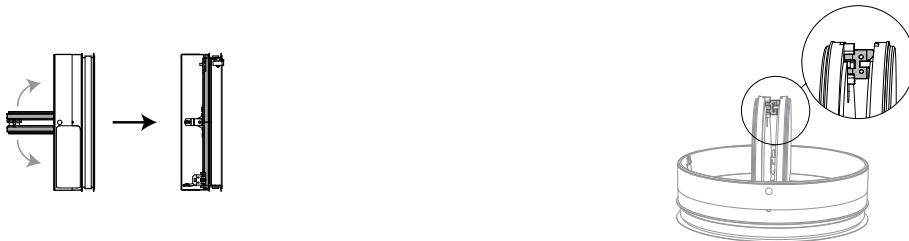
Unlock (close) the damper blades by pushing them towards each other. Carefully unlock the fusible link by pushing it sideways.
